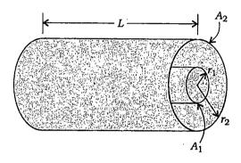
where 1 stands for inner cylinder and 2 stands for outer cylinder.
