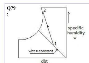
Which one of the following statement is correct for a cooling and humidification process 1-2 as shown on the psychometric chart shown in figure?
