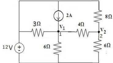
$$A = \frac{V_2 - V_1}{4} + \frac{V_2}{8} = \frac{V_2}{6}$$
