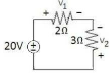
$$|V_1 = 8V, V_2 = 12V$$
